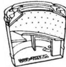
The Duo-Therm Burner transfers more heat to your home *quicker*, because its full-bodied, mushroom type flame floats in the lightweight steel heat chamber . . . *hugs* the chamber walls. There are no moving parts—nothing to wear out. And it's utterly silent!
